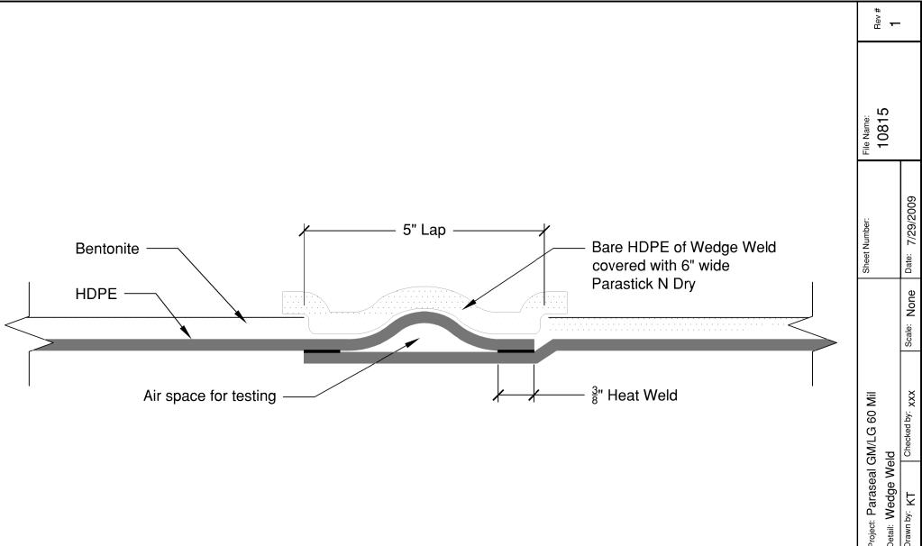
Note: Paraseal products require a minimum 24 psf compaction/ confinement in order to function as designed
